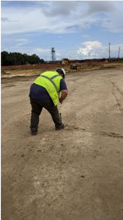
Photo 1.4: First preliminary Nuclear Gauge Density Test.
